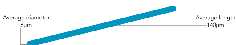
Figure 5: Optimised fibre aspect ratio
