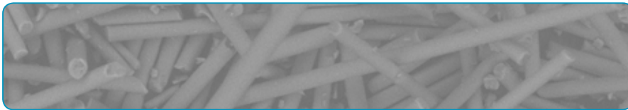
Figure 1: Raw short glass fibres used in everX Flow
